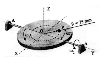
velocity and acceleration of particle P at the instant when the platform is in the XY plane and radius vector to the particle forms an angle of 60° with the Y-axis as shown.
