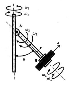
bearings at B due to the motion at a time when  $\theta = 60^{\circ}$ ? Take  $\omega_1 = 4 \text{ rad/}s^2$ ,  $\omega_2 = 3 \text{ rad/}s^2$ ,  $\omega_3 = 2 \text{ rad/}s^2$ .
